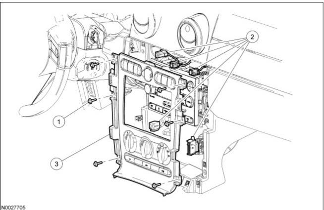
ItemPart NumberDescription1W705314Instrument panel center finish panel screw (6 required)2—Instrument panel center finish panel electrical connectors (5 required) (part of 14401)36304302Instrument panel center finish panel
